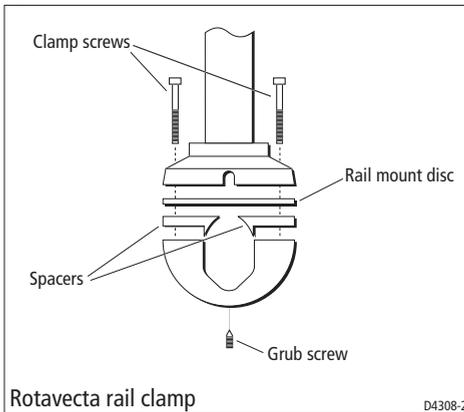
2. If the rail is 1 in (25 mm) diameter, set aside the two spacers. If the rail is between 0.9 in (23 mm) and 1 in (25 mm) diameter, place the spacers in the lower part of the clamp.
