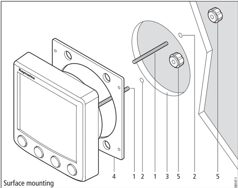
2. Apply the surface mount template (supplied at the rear of this handbook) to the selected location and mark the centers for the fixing studs (1) and the aperture (3) that will take the rear casing of the instrument.
