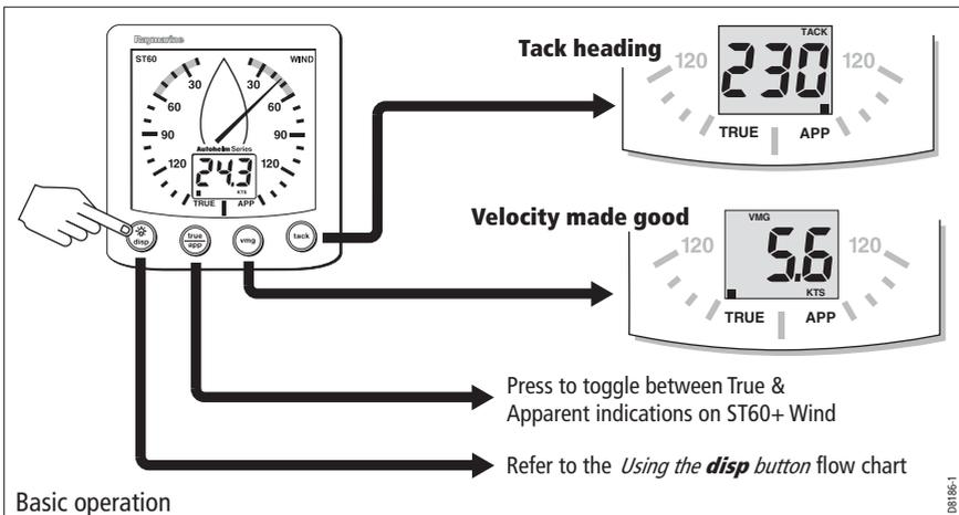
Use the *Basic operation* and *Using the disp button* flow charts in this Chapter, to operate your ST60+ Wind and ST60+ Close Hauled Wind instruments.
