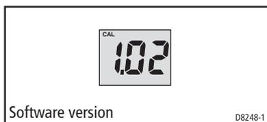
2. Note the software version number, then hold down the **disp** and **true/app** buttons for approximately 2 seconds, to return to normal operation.
