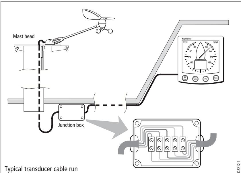
Typical transducer cable run
