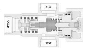
**NOTE!** In order to obtain a correct mix, the pressure of the hot and cold water must be the more or less the same.
