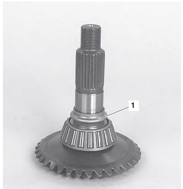
57. Remove the ferrule (1) from the output shaft.
