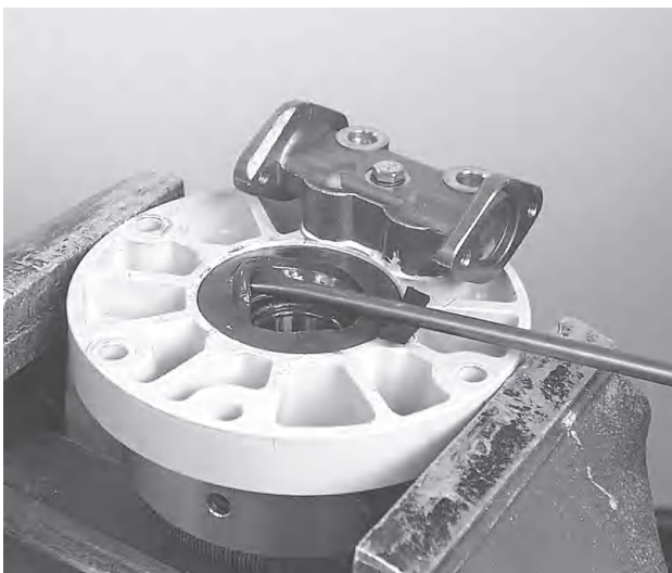
55. Remove the seal ring. Use a screwdriver or similar tool.
