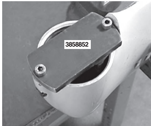
8. Lock the pinion nut with tool no. 3858852 . Press the shaft down and make sure that the pinion nut engages in the tool. Fix the tool to the rear bearing housing, using socket cap screws.
